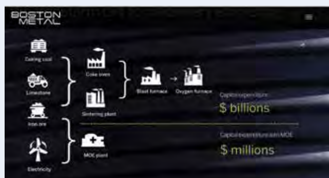
Image 3: Molten Oxide Electrolysis process versus conventional steel process.
